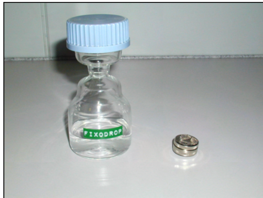
Suitable bottle and basket for immersing items in Fixodrop
